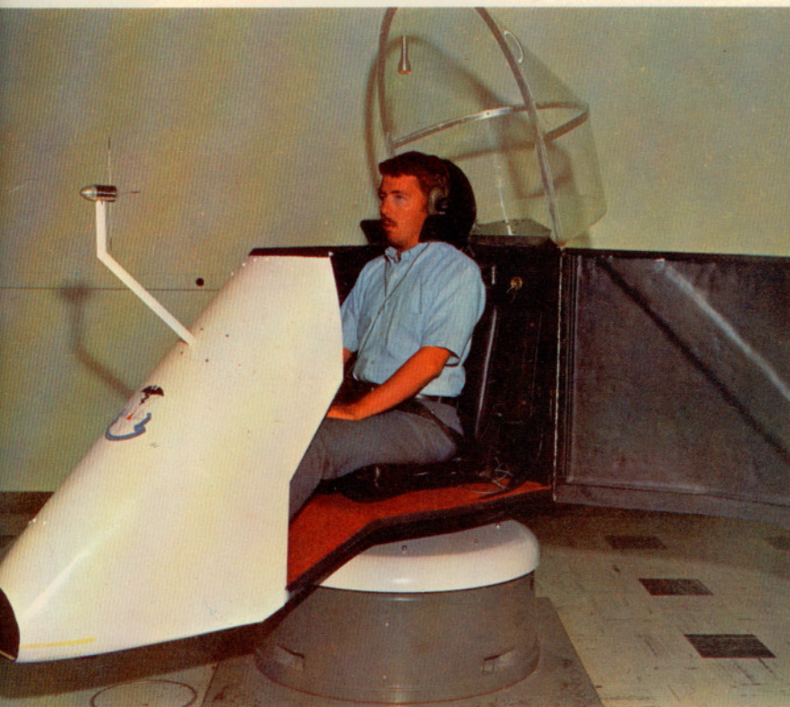
David Schroeder of the FAA Psychology Laboratory is seated in the CAMI disorientation device, which has been used in a number of research projects. Among studies currently in progress are those examining the effects of alcohol on blurring eye movements and the sensations of vertigo.
